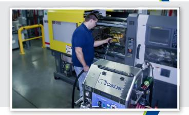
"CLEANING WITH COLD JET WILL NOT ROLL PARTING LINES, CHANGE OR DESTROY THE METAL AND BEST OF ALL, IT ALLOWS OUR RUNNING TIME TO BE EXTENDED. WE USE IT EVERY DAY, ON EVERY SHIFT."
