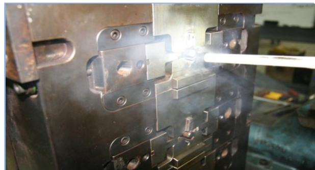
Fig 12 – In-Machine mold cleaning photo
