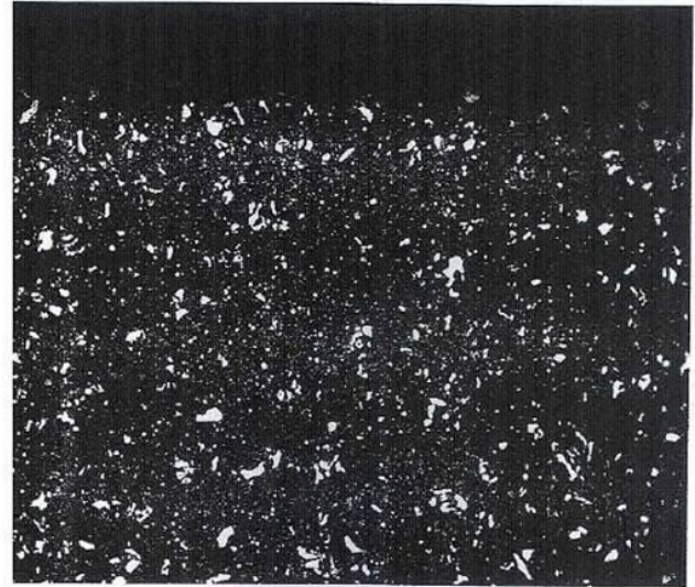
Fig. 9 – Unaltered carbide particles after cleaning
