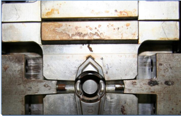
Fig. 13 – Off-gassing clogging the vent area (before photo)
