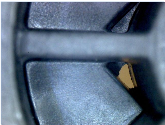
Fig. 15 – Before photo of PEEK part flash
