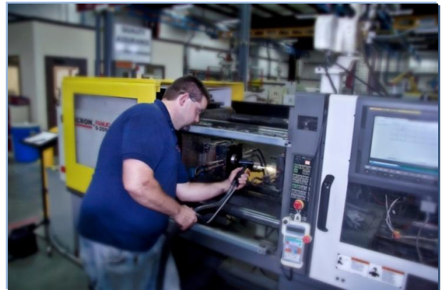
Fig. 11 – In-Machine mold cleaning photo
